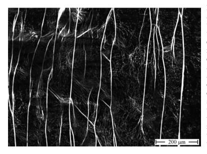
Fig. 1: Panchromatic cathodoluminescence map of a wafer cut perpendicular to the growth direction. Bright lines indicate LAGBs, points indicate single dislocations.
